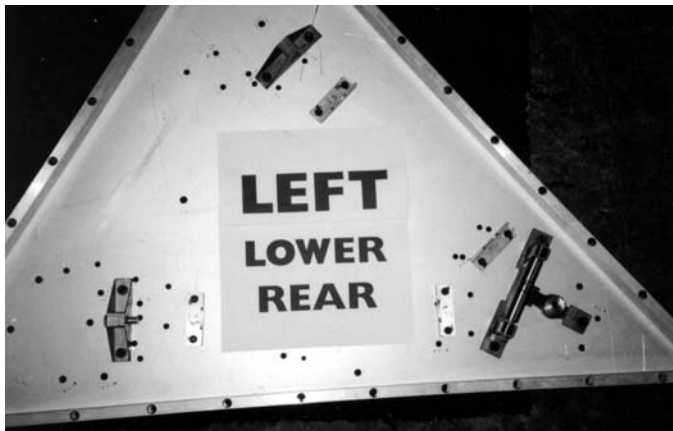
Figure 6-22 – This portable jig was set up to build all the upper and lower A-Arms for a formula car. One side was designed for the left side suspension while the other side was used for the right side suspension.
